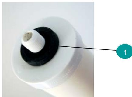
6. Check the new cartridge and the sealing washer (1) is correctly positioned. Check that the 'O' Seal inset in the top of the head (2) is correctly positioned. Screw the cartridge into the head until you feel the resistance of the washer meeting the sealing face. Continue to screw the cartridge a further ¼ turn to make an effective seal. **Important note.** Do not be tempted to over tighten the cartridge; over tightening will distort the sealing ring.
