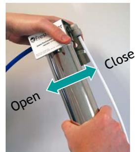
4. Lift the housing assembly off the retaining screws and holding the head firmly with one hand carefully unscrew the filter sump until it is free from the head. Empty the water from the filter sump and put the sump to one side.
