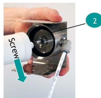
7. Tighten the sump firmly to make a watertight seal. Turn on the water supply and check the system for leaks. Leave the tap in the on position and allow the water to continue running for a minimum of 5 minutes to flush the cartridge. Your filter system is now fully operational and ready for use.
